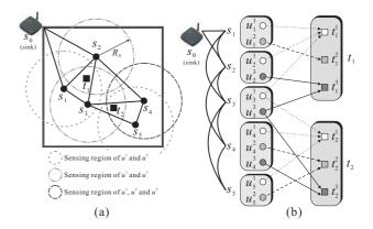
An illustrated example: (a) the topology, (b) the coverage and Fig. 1. connectivity relationships.
